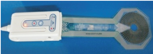
(c)压力薄膜传感器
